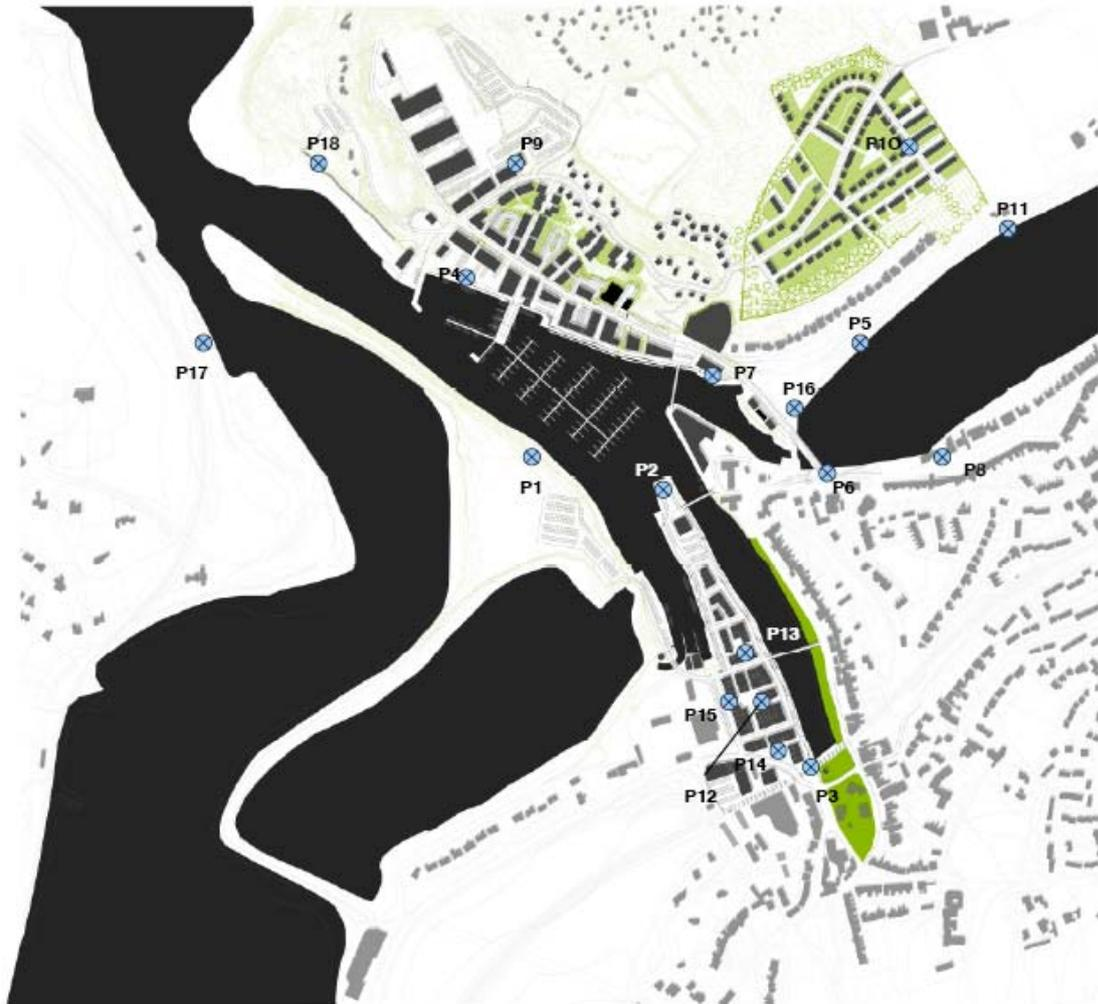
Figure 6– 2 Noise survey measurement positions
